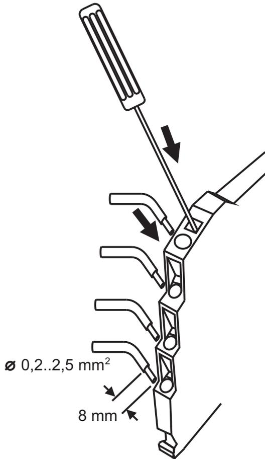
The module has been designed for spring-type terminal electrical connections.
