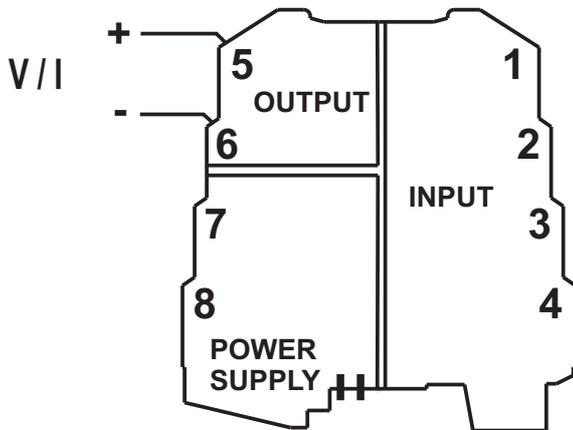
Note: in order to reduce the instrument's dissipation, we recommend either using the output for voltage or guaranteeing a load of  $> 250 \Omega$  to the current output.
