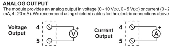
There is no insulation between RS485 and the analog output.
